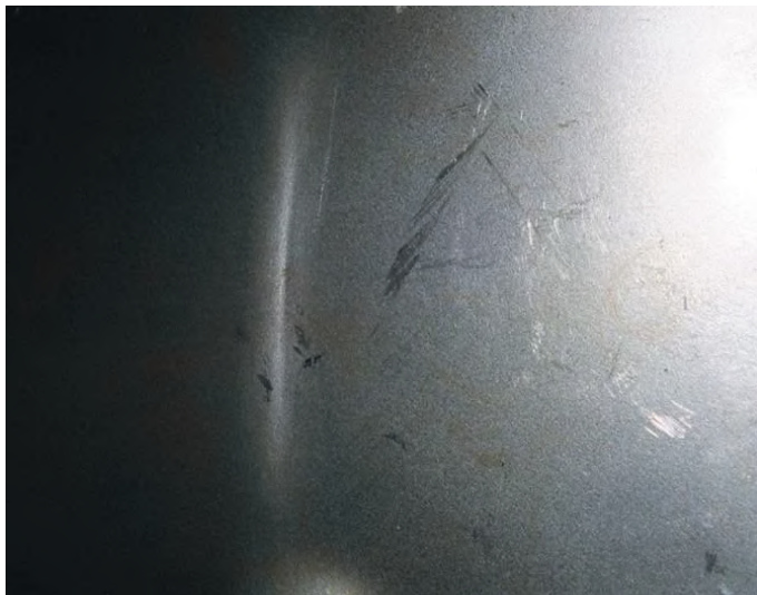
Figure D.2 — Typical YPE strain lines in carbon steel
