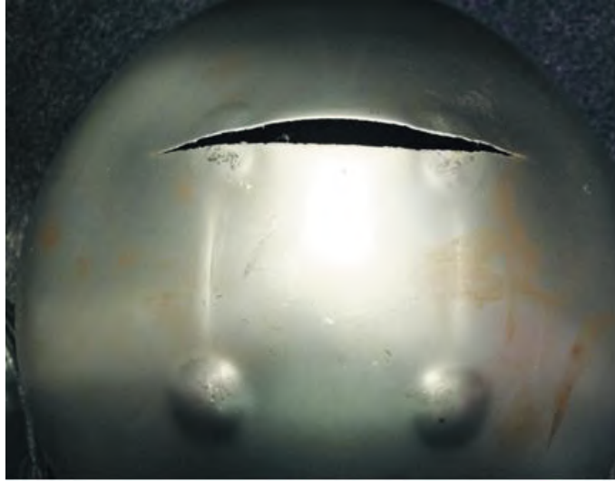
Figure D.4 — Example of YPE strain lines and YPE fracture
